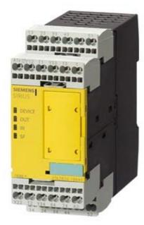
SIRIUS SAFETY RELAY WITH RELAY RELEASE CIRCUITS (RC), DC 24V, 45.0MM, SPRING-LOADED TERMINAL, RC INSTANT.: 4S, RC DELAYED: 0, MK: 3, 8-FUNCTION SWITCH, BASIC DEVICE, MAX. ACHIEVABLE PL TO EN13849-1: E, MAX. ACHIEVABLE SIL TO IEC61508:3,
