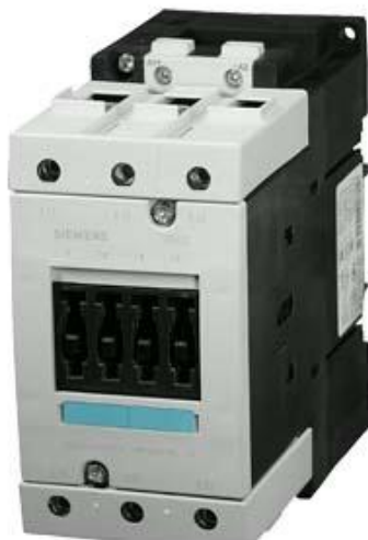
CONTACTOR, AC-3 37 KW/400 V, DC 24 V, 3-POLE, SIZE S3, SCREW CONNECTION
